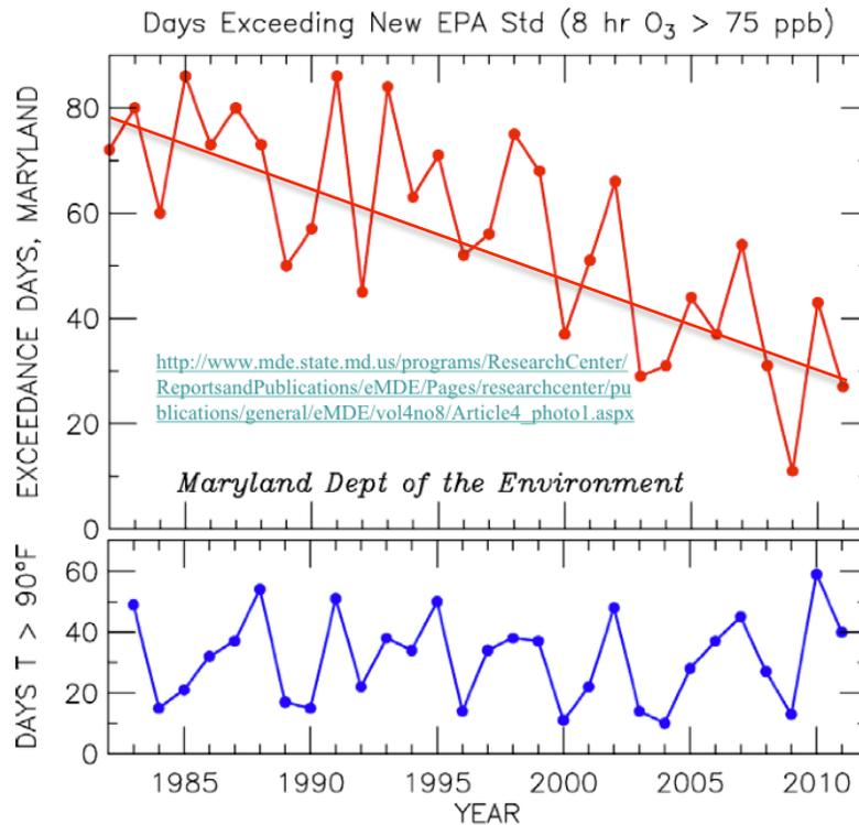
Figure 3. Data from the Maryland Department of the Environment (MDE) showing the number of O<sub>3</sub> exceedance days per year and temperature at the BWI airport above 90° F. Adapted from Ross J. Salawitch
