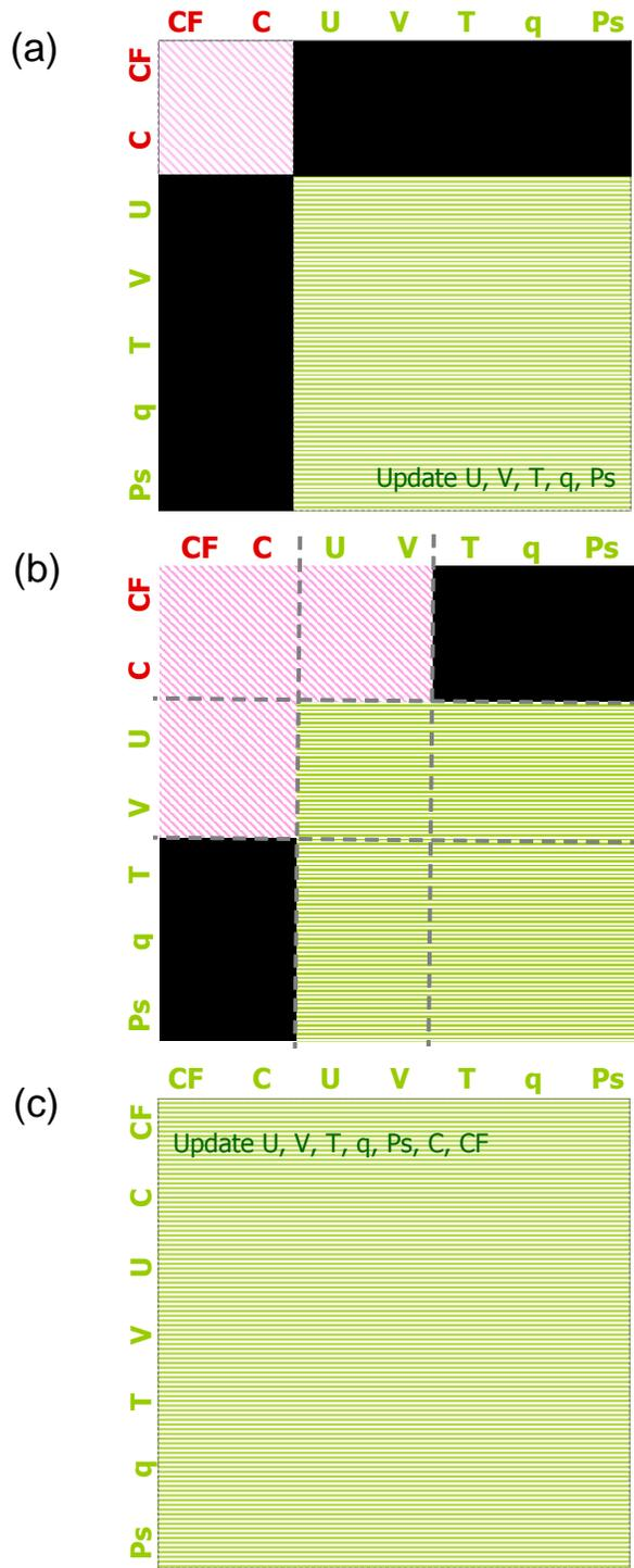
Figure 2. 1. Schematic plots of the background error covariance matrix for (a) C-univariate, (b) 1-way multivariate, (c) multivariate data assimilations. (C: atmospheric CO<sub>2</sub>, CF: surface CO<sub>2</sub> fluxes)
