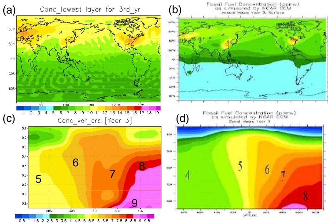
**Figure 2. 5. Comparison of SPEEDY-C with NCAR CCM: annual mean of atmospheric CO<sub>2</sub> concentration in the surface layer for third year in (a) SPEEDY-C, and (b) NCAR CCM, and the vertical cross section of zonal mean at the beginning of 3<sup>rd</sup> year simulation in (c) SPEEDY-C, and (d) NCAR CCM. The experiment starts from zero state of CO<sub>2</sub> in the atmosphere with a fossil fuel emission of 6 PgC/yr. (unit: ppmv)**
