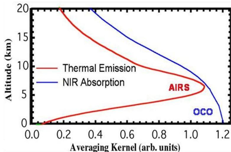
**Figure 2. 4. Representative vertical averaging kernels for column CO<sub>2</sub> soundings using near IR absorption of reflected sunlight in the 1.61- $\mu$ m CO<sub>2</sub> band (blue) and thermal IR emission near 14.3  $\mu$ m (red). Thermal IR soundings are less sensitive to near-surface CO<sub>2</sub> because of the small surface–atmosphere temperature contrast. (Crisp et al., 2004)**
