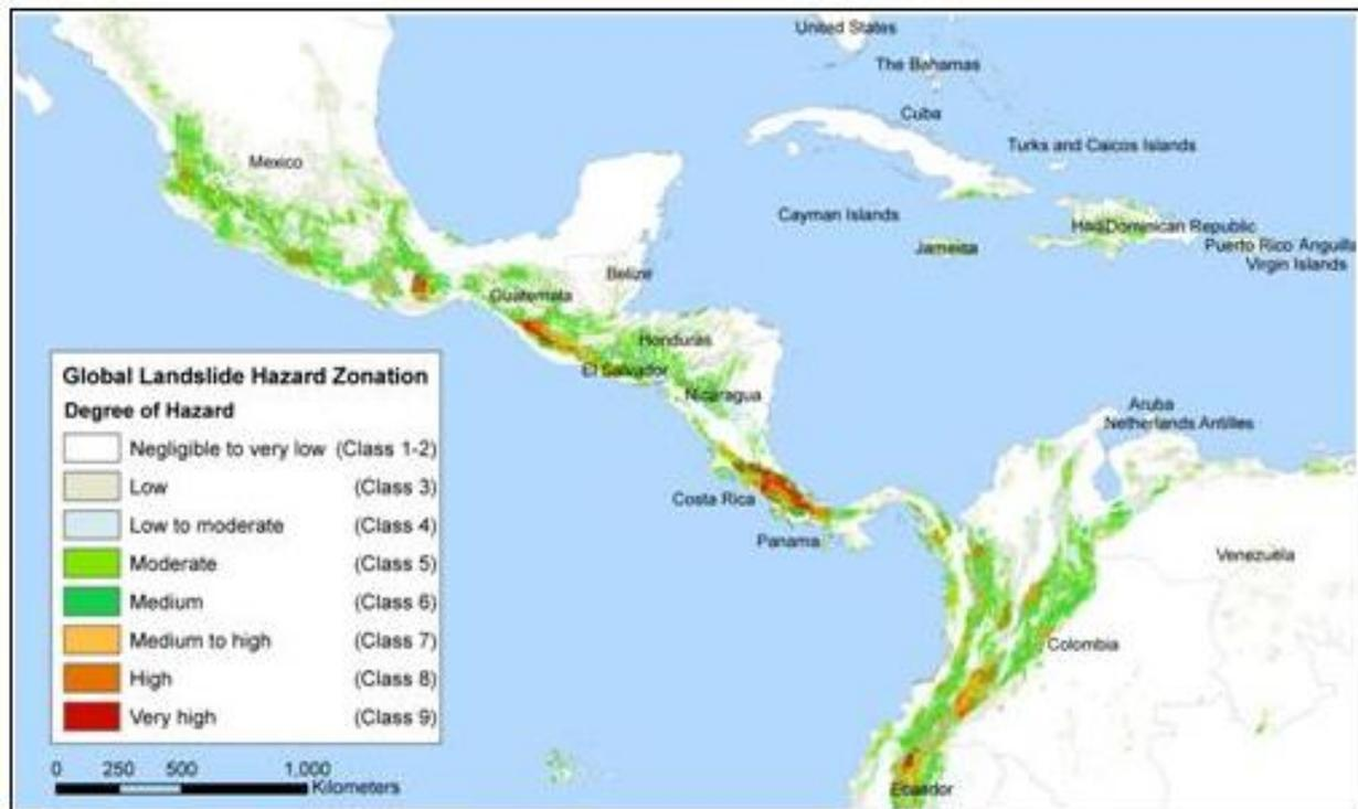
**Figure 1.2.** Landslide hazard zonation in Central America and northwestern South America. Figure adapted from Nadim et al. (2006).
